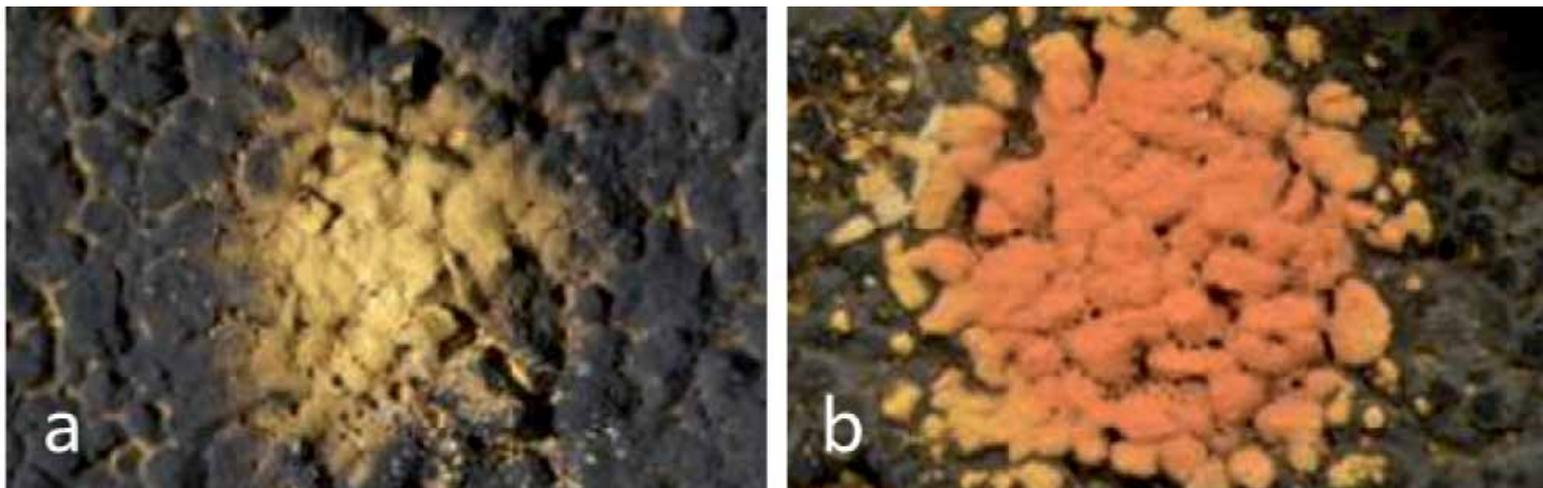
Fig.2 - Microscope images (magnification 7x) of the soot removal with a) Kinpen (20 minutes) and b) PlasmaPen (40 seconds). The colour change using PlasmaPen is clearly visible
