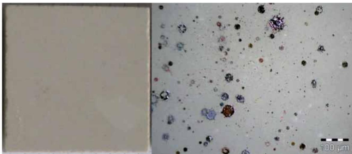
Fig. 1 - Picture of Istria Limestone after the plasma treatment with Blaster from Tigres Dr Gerstenberg GmbH (left) and optical microscopy image of the surface after a treatment of 600 sec. with the same equipment (right)
