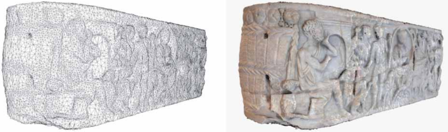
Fig.5 - The wireframe 3D model and the mesh with texture of the sarcophagus
