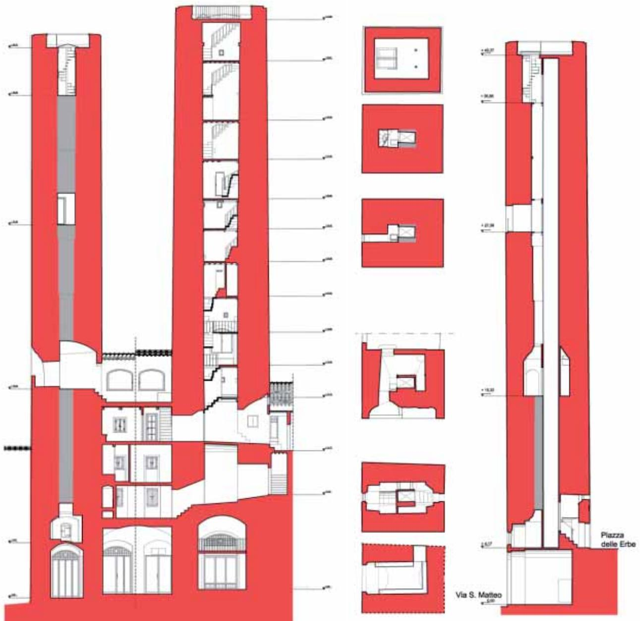
Fig.4 - Longitudinal section of the Salvucci Towers (the North tower is on the left); Fig.5 - Cross-section of the North Salvucci Tower and plans at the six levels marked in the section
