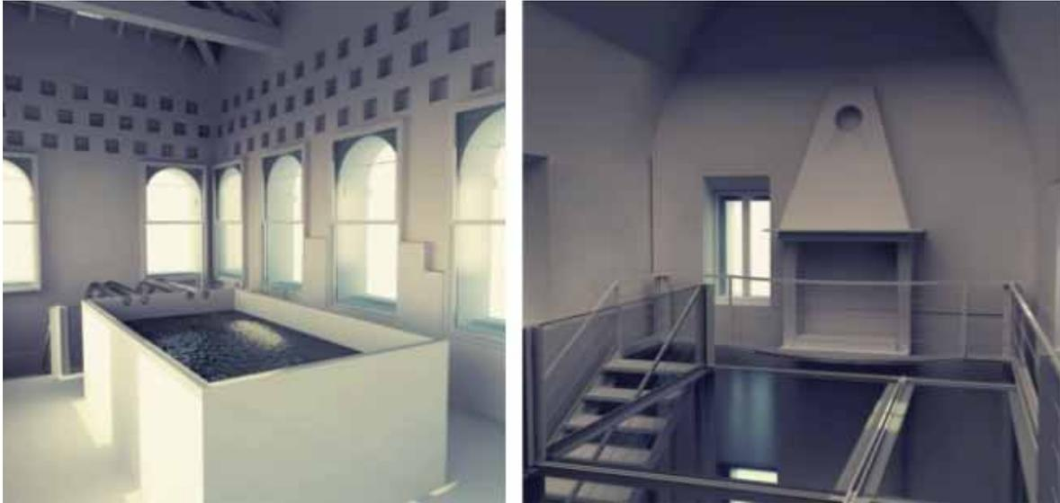
Fig.7 - On the left, the designed great cistern, repositioned at the extrados of the vault, after the restoration of the roof. On the right, some internal views, after the intervention, of the steel structure inserted in the unique original volume of the tower
